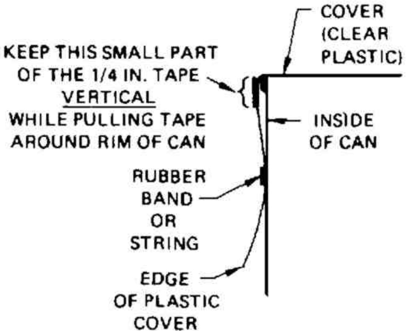
4. Make the cover so it fit snugly, but can be taken off and replaced readily.
