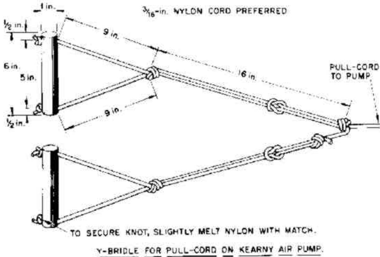
A man of average size and strength can operate a 6 ft X 29 in. KAP by himself, pumping over 4000 cubic feet per minute through a typical large shelter without working hard; tests have shown that he must deliver only about 1/20 of a horsepower. However, most people prefer to work in pairs when pulling a 6-ft KAP equipped with a "Y" bridle, when pumping over 3000 cfm.
