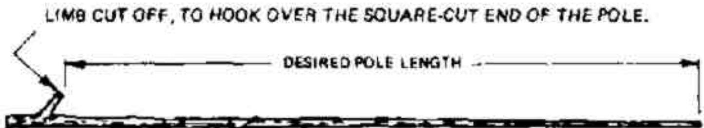
(5) It usually is best first to cut the poles exactly two or three times the final length of the poles to be used in the shelter.
