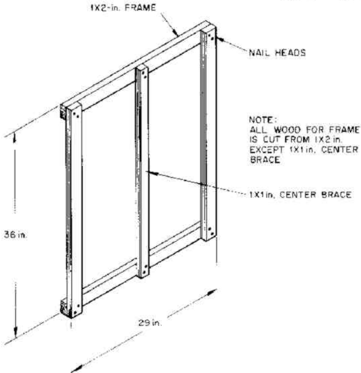
b. To make the front side smooth and flat so that the flaps will close tightly, fill in the spaces as follows: Cut two pieces of 1 X 2-in. boards long enough to fill in the spaces on top of the 36-in. sides of the frame between the top and bottom horizontal boards, and nail these filler boards in place. Do the same thing with a 1 X 1-in. board (or a board the size of that used for the center brace) as a filler board for the center brace (see Fig. 4).
