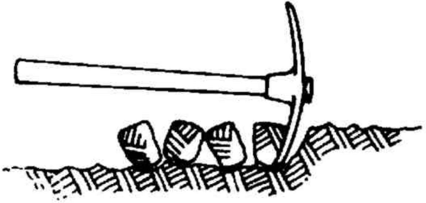
9. When digging a trench, to avoid having to move the excavated earth twice more to get it out of the way, first pile all earth about 8 ft away from the trench. Later, pile additional earth you are excavating at least 3 ft away.
