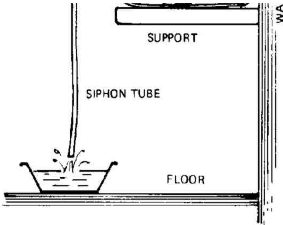
Water can be siphoned from a covered water storage pit into a belowground shelter so that the siphon will deliver running water for weeks, if necessary. The Utah family mentioned earlier siphoned all they needed of the 120 gallons of water stored in a nearby lined pit. A field-tested method of siphoning follows:
