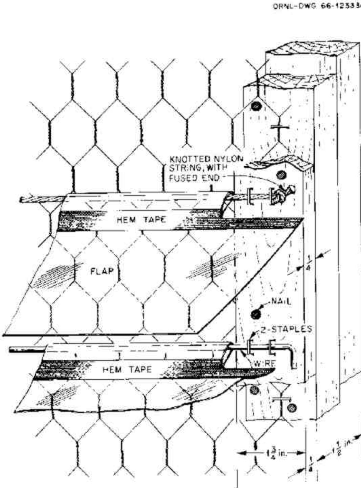
Note in Fig. 13 that each pivot-wire is held firm and straight by 2 staples securing each end. The wire used should be at least as springy as coat hanger wire. If string is used instead of wire, nylon cord about the diameter of coat hanger wire is best for the pivot-strings.
