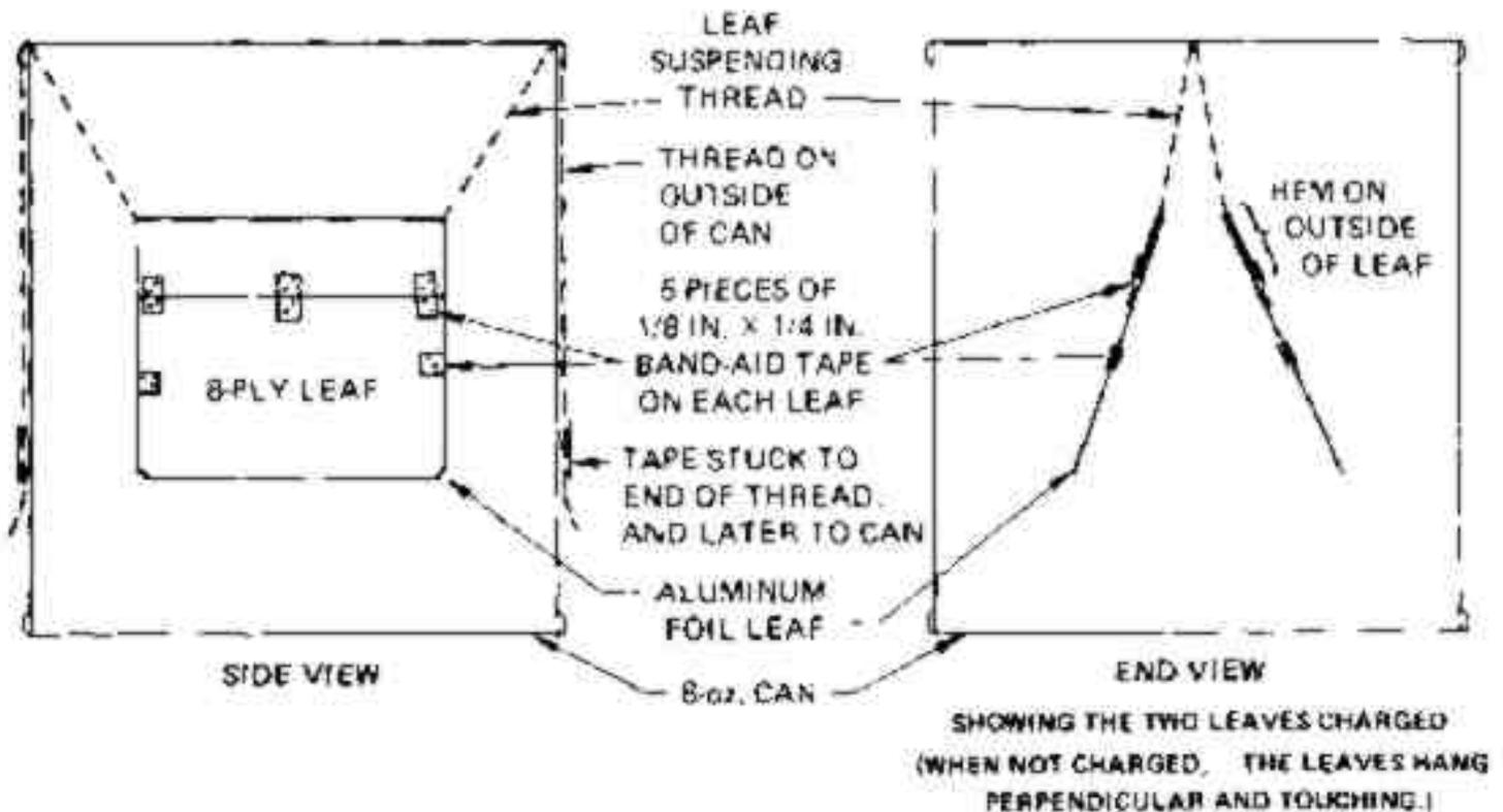
19. To prevent possible partial discharge from overly sharp lower corners of the leaves, use scissors to cut about 1/16 inch ( L ) off each lower corner of the two leaves. (Partial discharge from an overly sharp corner may prevent a KFM's leaves from being adequately charged and adequately separated.)
