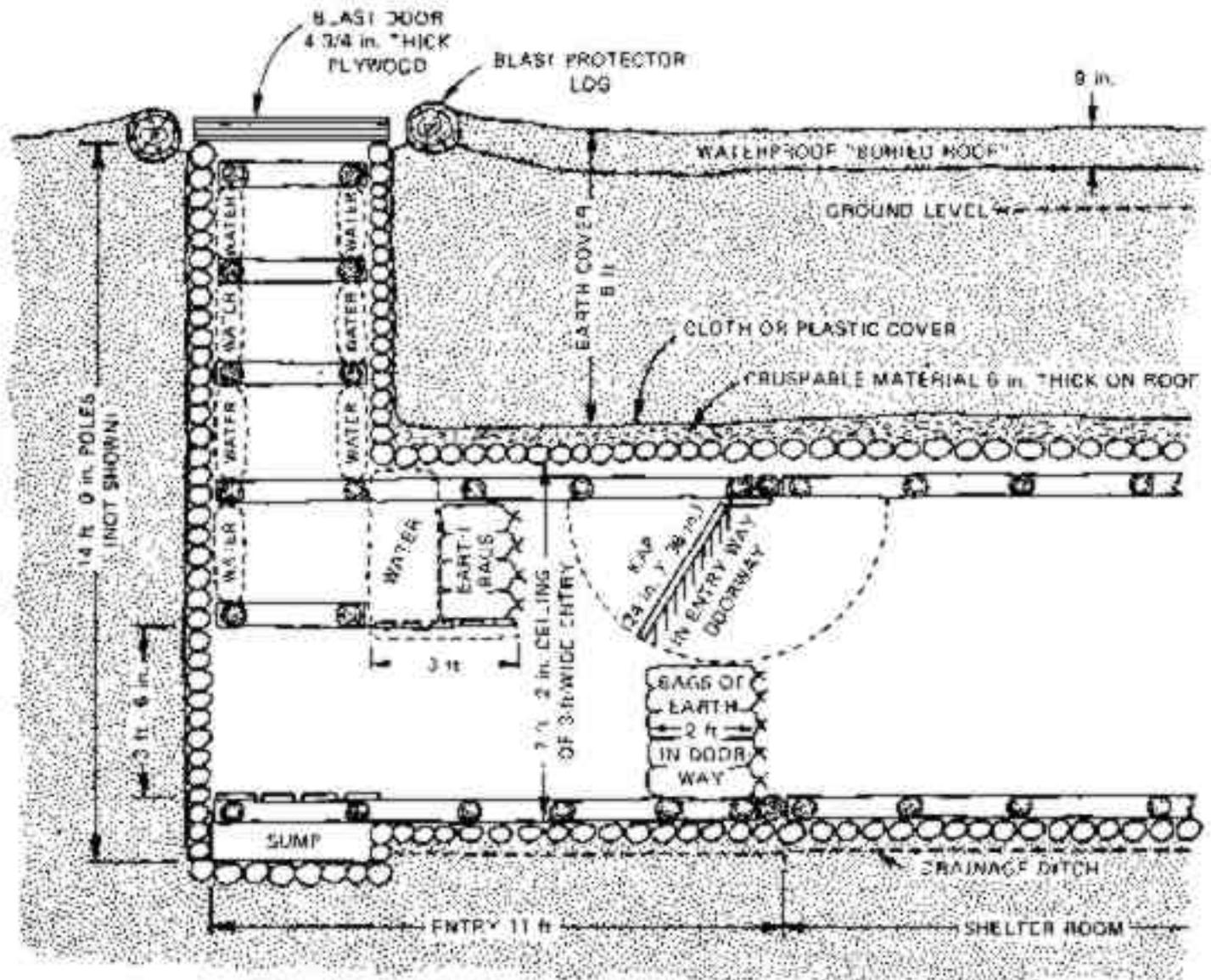
° Made with 4 rectangular horizontal braces in each vertical entry, in addition to the ends of the two long, ladder-like braces. The detailed drawings in Appendix A show such braces. The lowest rectangular brace should be positioned 3-1/2 feet above the flooring at the bottom of the vertical entry (see Fig. D.20).
