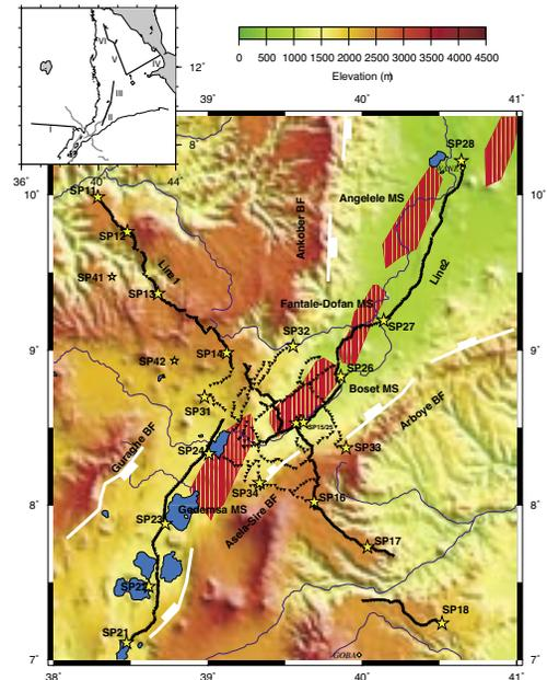
Figure 1: Index map of the EAGLE controlled source experiment. Line 1 crossing the rift valley; Line 2 follows the rift valley; and Line 3 is the array deployed in the region where Lines 1 and 2 cross. Yellow stars are shotpoints. Elongate areas shaded in red are magmatic segments that were targeted in this study. The inset shows the locations of previous studies in the region.
