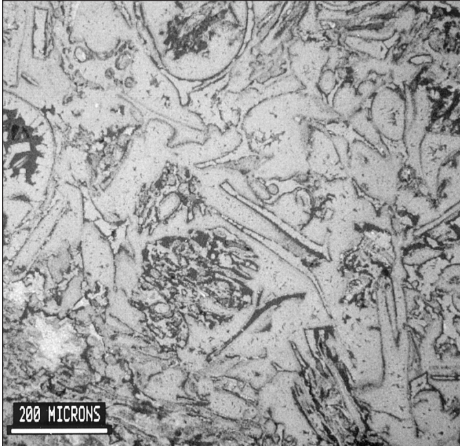
Figure 5. Typical bentonitic ash from the Middle Awash. This 30-cm-thick altered tuff is interbedded with bentonitic clastic sediments. The tuff is completely bentonitic, but relict textures are excellent. It was an ash fall bed that was altered in situ . Leaching during hydrolysis of the glass was responsible for the reduction of porosity. The relict textures indicate that the ash fallout consisted of large, thin-walled (10–30 \mu\text{m} long), elongate, straight, slightly curved platy shards. These are also some hollow spheres. The ash also contained ~25% equant, 100–200- \mu\text{m} -wide, angular pumice clasts (up to 2 mm long). The tuff is nearly aphyric, with only traces of very small, angular sanidine phenocrysts. Compare with the unaltered ash in Figure 4A.
