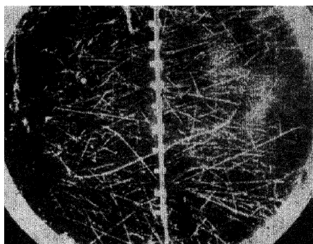
Fig. 6. Cloud chamber picture showing both recoil fragment tracks of a fission originating on the foil. The cloud chamber was filled with argon and water vapor to a pressure of 20 cm and the mica foil was 1.2 mg/cm 2 thick. (Bøggild, Brostrøm and T. Lauritsen).
