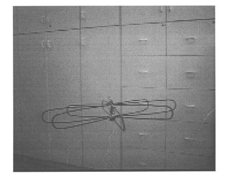
Above: The oscillator/tank circuit assembly hung as a pendulum on a very thin twin wire, carrying the DC supply to the circuit.
