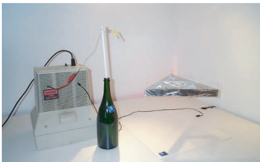
FIGURE 248 Lifting a light object – covered with aluminium foil – using high a tension discharge (© Jean-Louis Naudin at http://www.jlnlabs.org )
