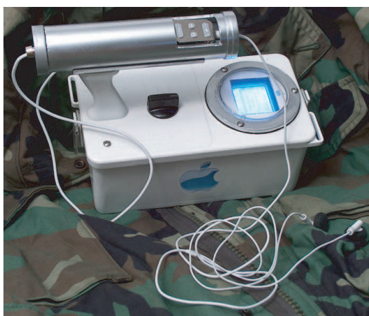
FIGURE 374 A Geiger–Müller counter with the detachable detection tube, the connection cable to the counter electronics, and, for this model, the built-in music player (© Joseph Reinhardt)
