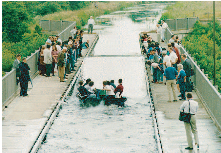
FIGURE 112 A solitary water wave followed by a motor boat, reconstructing the discovery by Scott Russel (© Dugald Duncan)
