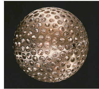
FIGURE 197 The LAGEOS satellites: metal spheres with a diameter of 60 cm, a mass of 407 kg, and covered with 426 retroreflectors (NASA)
